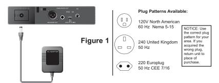
Connect the AC/DC adapter cable to the DC 12V input jack. Then plug the adapter unit into an appropriate AC outlet as shown in Figure 1.
